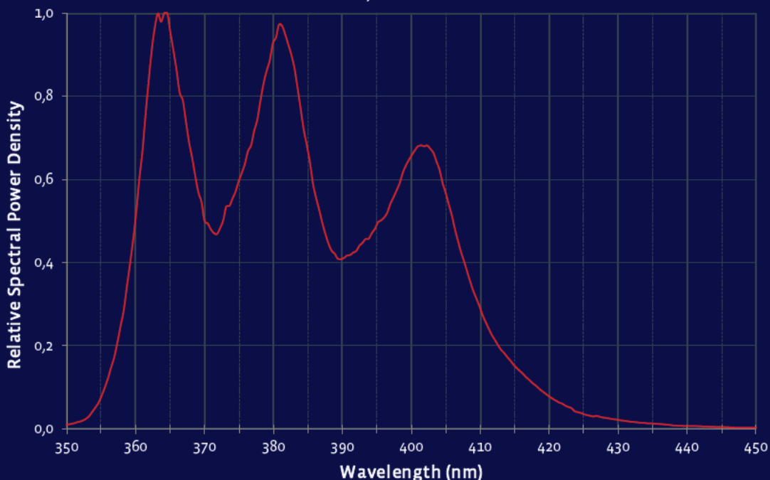
Triple Wavelength Configuration: Spectral Power Distribution 365 nm , 385 nm and 405 nm
