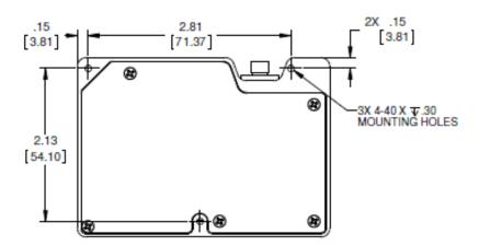
**Figure 1: Flame-NIR Outer Dimensions**
