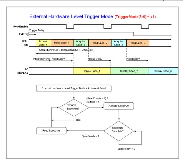
**External Hardware Level Trigger Mode Timing Sequence**
