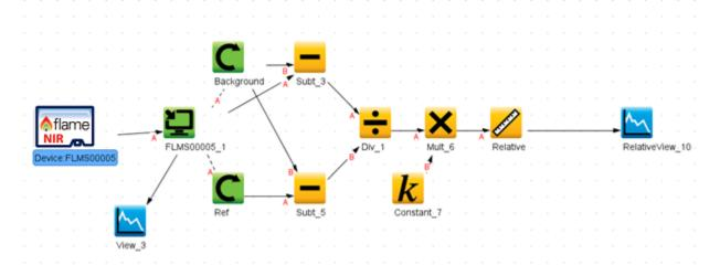
The schematic view is a graphical interface that allows you to move from device through to processed data. There are a few basic components to consider.
