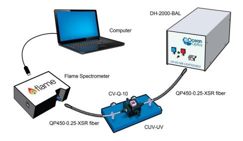
Ocean Optics Flame-NIR Fiber Optic Spectrometer Typical Set-up
