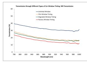
Figure 5. Effective blocking of heat-generating Vis-NIR radiation is one of the key functions of tinting in car windows.
