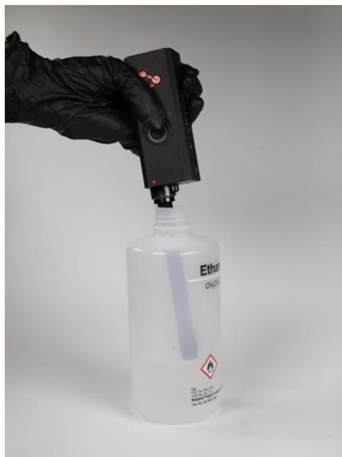
As result a novel optics miniaturization strategy allows us to create **compact Raman spectrometers and microscopes** based on non-stabilized laser diodes, densely-packed optics, and non-cooled small pixel size sensors.
