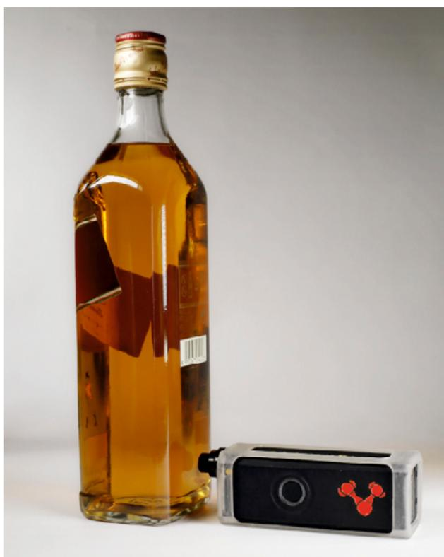
Figure 1. Photograph of miniaturized Raman spectrometer measuring whiskey content through the glass bottle
